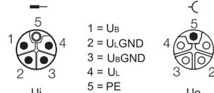
注: U<sub>B</sub>为模块电源, U<sub>L</sub>为负载电源;
