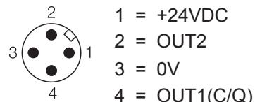
Note: OUT1: switching signal or IO-Link
