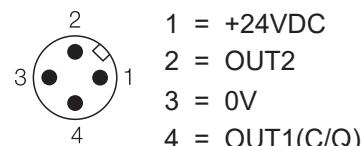
Note: OUT1: switching signal or IO-Link
